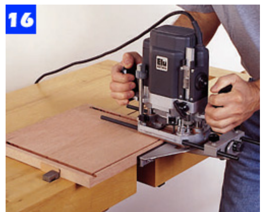
After routing the dovetail slots in the drawer fronts and sides, use a 1/4-in. straight bit to rout the bottom groove.
