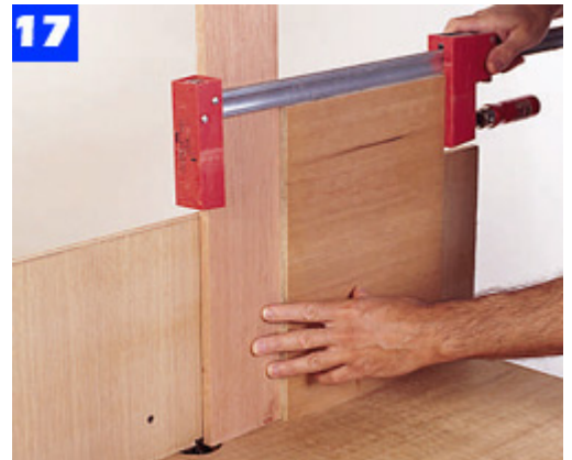
17 Install the dovetail bit in your router table and cut the dovetails on the sides and backs. Then, test fit the joints.
