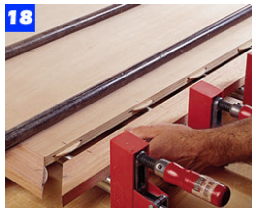
18 Use plate joints to assemble the top panel and mitered mahogany edging. Panel top is 1/16 in. below top of edging.
