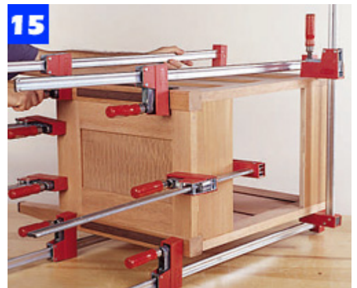
Apply glue, and clamp together the front leg/panel subassembly and the side-panel subassembly. Let the glue set.
