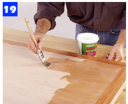
19 Brush two coats of wallpaper adhesive onto the desktop panel, paying extra attention to the edges and corners.
