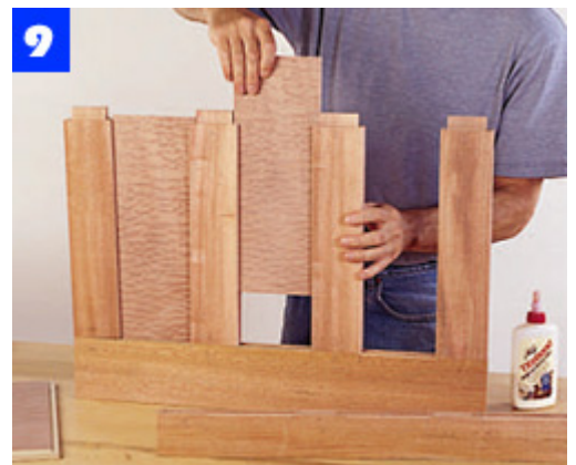
Apply glue and join the pedestal stiles to a rail. Slide the veneered panels into place and add the second rail.
