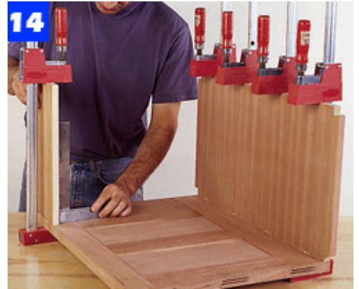
Join a case bottom and pair of stretchers to each pedestal side. Clamp, and check the assembly for square.
